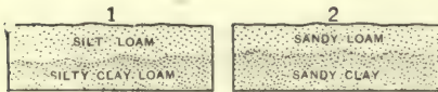
FIG. 104.—Soil and subsoil in (1) loess; heavy soil and a light soil are underlain by heavier subsoils.
